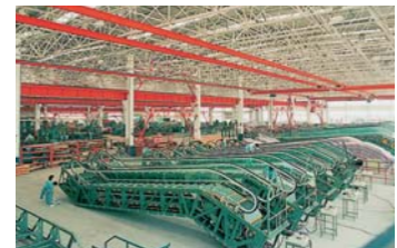
An escalator production line at Shanghai Huasheng Fujitec
